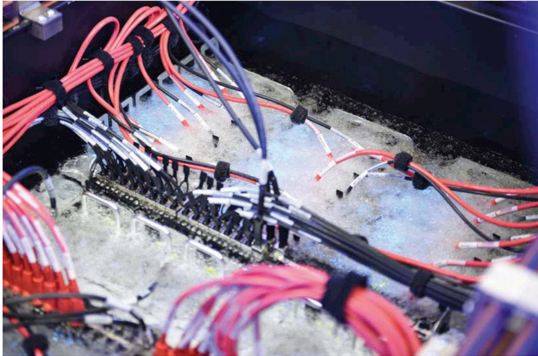
that fits around the lower half of the module, with an O-ring seal used to prevent leakage. Water is then pumped under the module when the car is running. Hitachi claims its approach cuts the junction temperature by 25°C compared to indirect cooling even using the same cooling fluid as that used for the main engine, which can be as hot as 105°C.
