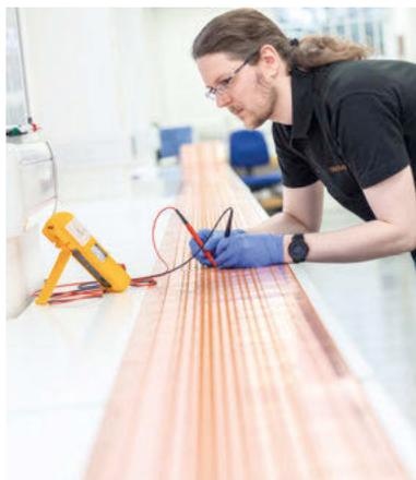
Left: Circuit inspection – checking for electrical isolation between tracks (Source: Trackwise)
