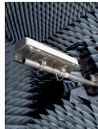
(Above) Cobham's antennas are tested in anechoic chambers.
