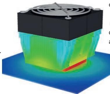
6SigmaET has been used to model a range of electronic designs, including DIMM arrays (top) and a processor heatsink
