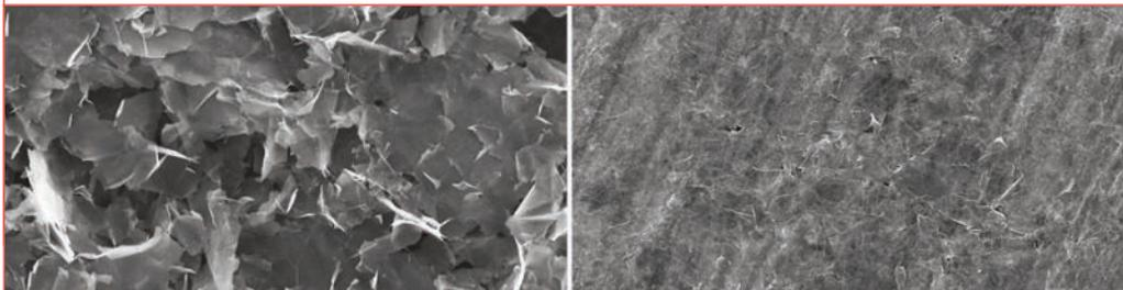
Electron microscope images show the graphene ink after it was deposited and dried (left) and after it was compressed (right)
